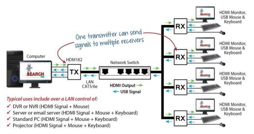
Note that when using on an office network, there may be network resource considerations, so in some instances it may be necessary to separate this functionality using a separate network switch.
