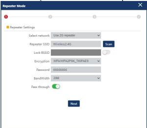
**Repeater SSID** is the WiFi network SSID this IPmitter is to connect to. To find the network you want to connect to press Scan and then select the WiFi network name.
