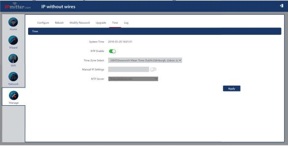
**Sync With Host** - Set the time to the same as computer time. This is only available if NTP is not enabled.
