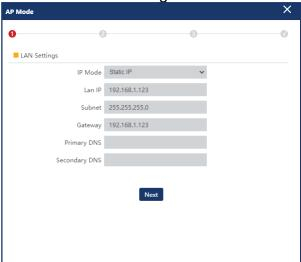
**IP Mode** can be set to either GHCP, static or DHCP. GHCP is set as standard, and will receive an address (similar to DHCP, but will also assign another IPmitter connected to an available address), static IP address is a unique fixed address which you can assign to the IPmitter. DHCP will obtain the address from the DCHP server or the router and assign IPmitter with an address from the network.
