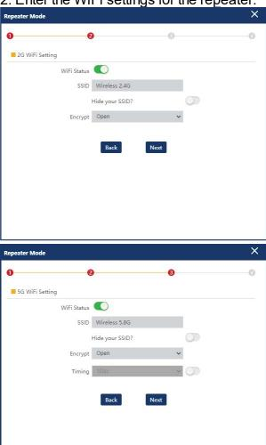
**WiFi Status** controls the WiFi on the repeater. When used purely as an IP camera bridge then it is recommended to leave this option off. When enabled the repeater will broadcast its own WiFi network as well as the existing WiFi network.
