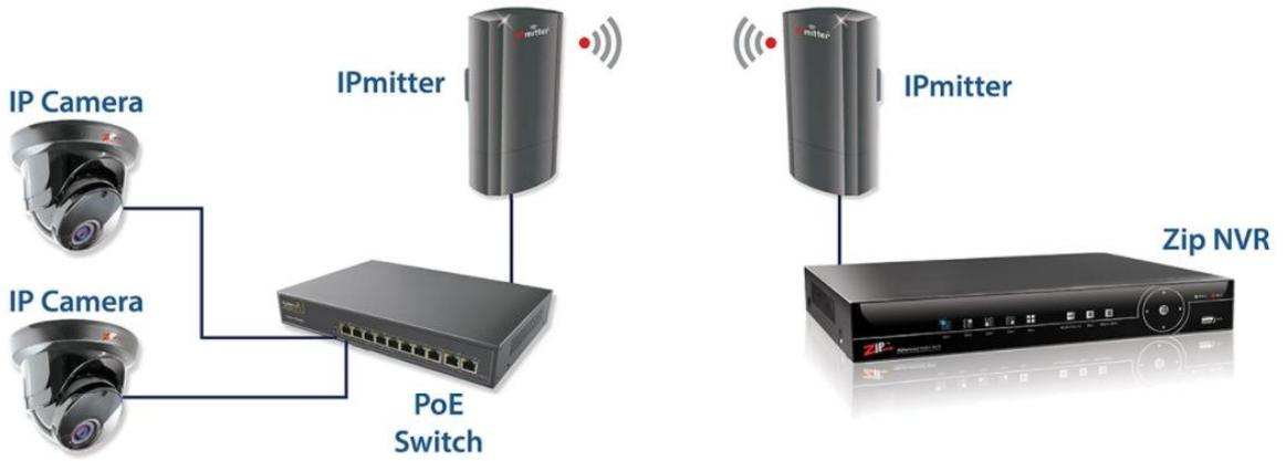
When pairing, one unit needs to be set to "Client" and the other unit needs to be set to "Host".
