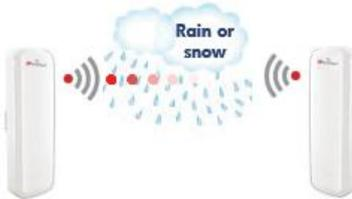
4. When installing the units in good weather the signal may be sufficient. However during heavy rain/ other poor weather the signals between the IPmitters will be absorbed, therefore reduce the distance achievable. Keep the distance between the two units as short as possible and within the recommended specification.
