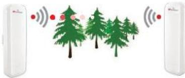
2. The may will go through branches of trees but remember that microwave signals will be attenuated greatly by water. Leafs and plants are partly made up of water so the distance is reduced. It is best to avoid plants and trees when positioning.
