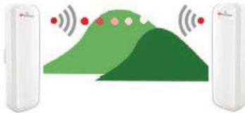
1. The Signal will no go through hills. The density of the hill and water contained in the soil absorbs the microwave signal.
