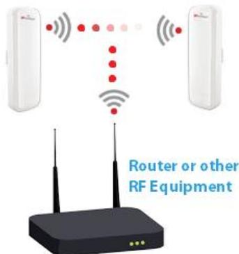
5. It is common that other RF equipment can interfere with the IPmitters, as the IPmitters use the same frequencies that routers and other WiFi equipment uses. This will reduce the range of the IPmitters and reduce the performance. Check the WiFi channels being used nearby to the IPmitter, or avoid placement of the IPmitters near other RF equipment and routers.
