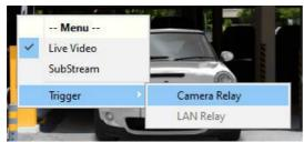
To enable "manual" triggering of an alarm, in this case the camera is configured as follows (In the cameras browser via Configuration > Alarm> I/O Alarm)..
