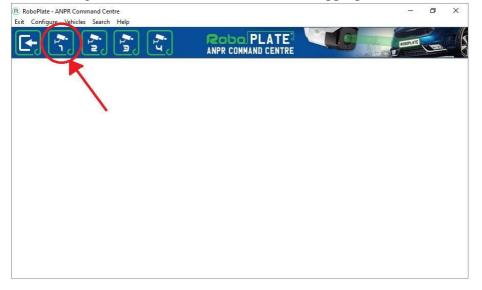
Individual listener windows open for each camera, they can be moved around screen or onto a secondary monitor, its position is saved when the window closes. If the window is out of sight, ie: not visible when opens, close it and open it again holding a shift key down whilst you do so.
