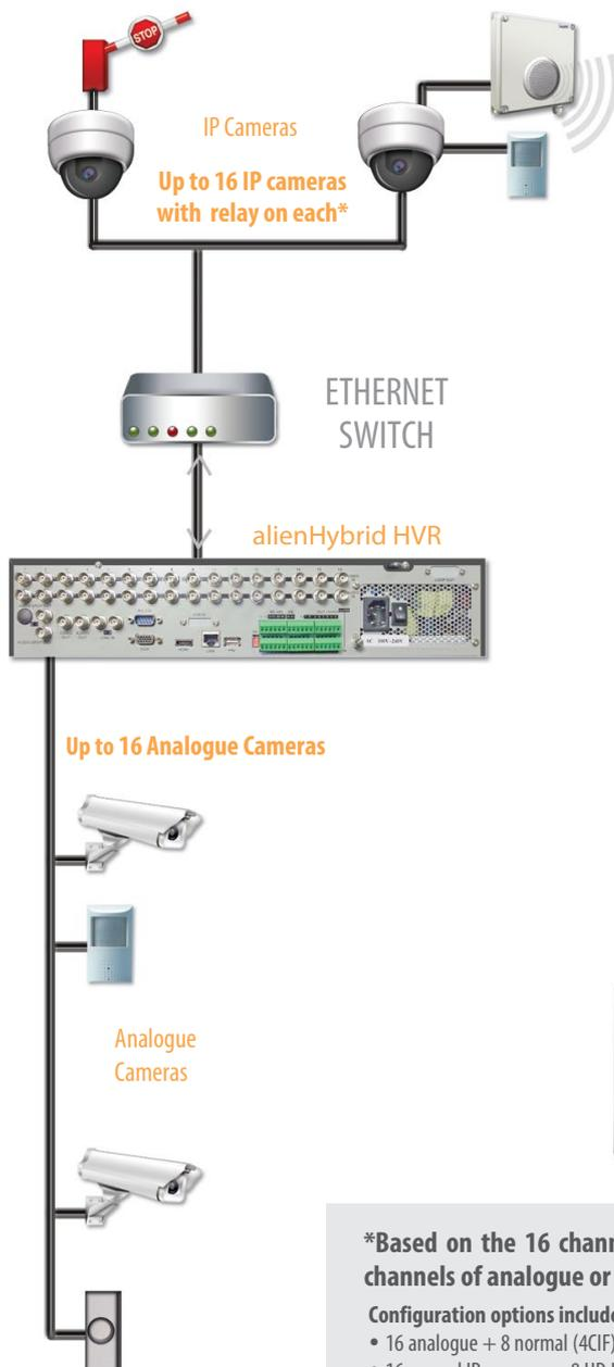
Each camera including any connected IP cameras can be linked to an alarm input such as a PIR, break beam, door contact or panic button to activate recording from that camera. An intelligent buffer system retains recorded footage from prior to the event occurring as well as for the pre-defined alarm time.
