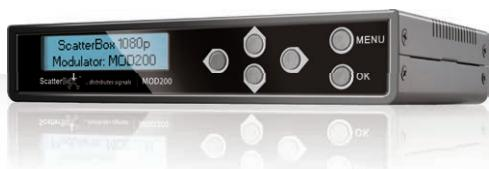
**Note:** The MOD200 has to process and digitise the HDMI input from the DVR and this creates a small delay or "latency" in its output, this is typically in the region of 200 milliseconds. This means the TV picture would be around 1/5 second behind what the DVR's output is doing. It's very similar to the latency you get with IP cameras systems.
