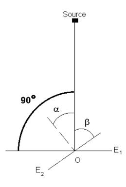
Effective illumination is proportional to the cosine of the angle of incidence of the light on the surface (angle between the direction of the light and the perpendicular to the surface)
