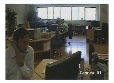
In this image with WDR switched off the buildings outside the window cannot be seen. The camera tries to take an exposure reading from the bright window area resulting in the rest of the image looking dark.
