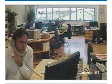
In this image with WDR switched on the buildings outside can be seen and the overall exposure of the resulting image has been improved.
